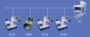
Thanks to its "Power over Ethernet" port, i3380 can be connected to an Ethernet LAN, reducing installation costs.
